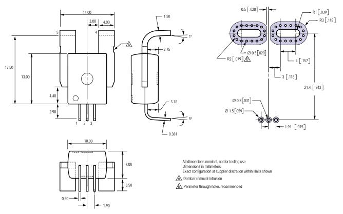
Creepage distance, current terminals to sensor pins: 7.25 mm Clearance distance, current terminals to sensor pins: 7.25 mm Package mass: 4.63 g typical
